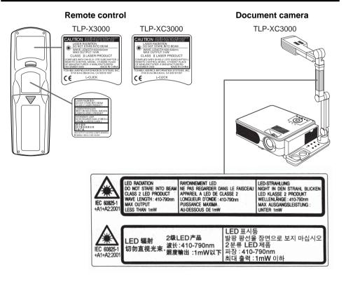
Caution - use of controls or adjustments or performance of procedures other than those specified herein may result in hazardous radiation exposure.
